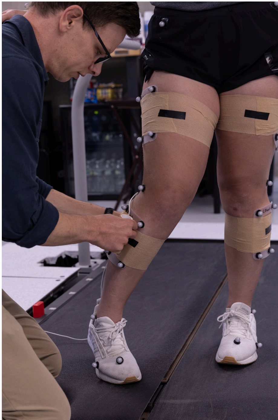
Uhlrich attaches the vibrating motors that provide real-time feedback to Miller to change her walking pattern. (Dan Hixson/University of Utah)
